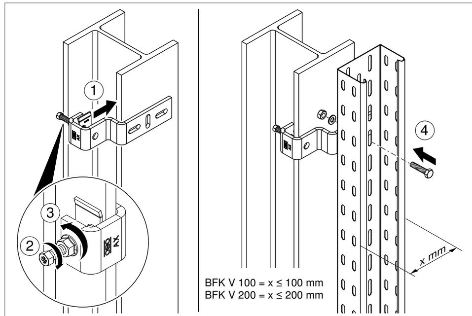
**Fig. 11:** Mounting a clamping piece on the exterior of a steel girder
