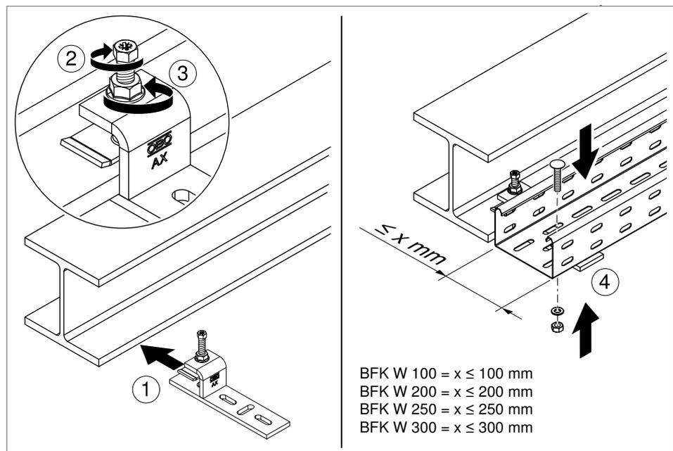
**Fig. 9:** Mounting a clamping piece on a horizontal steel girder
