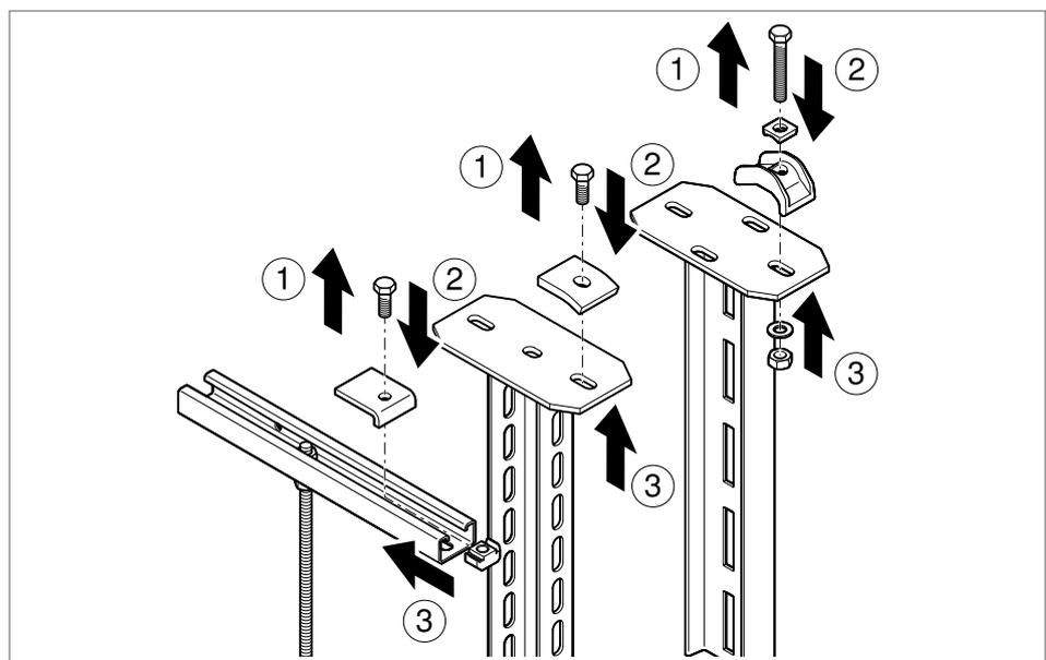
**Fig. 3:** Pre-assembling the clamp fastening
