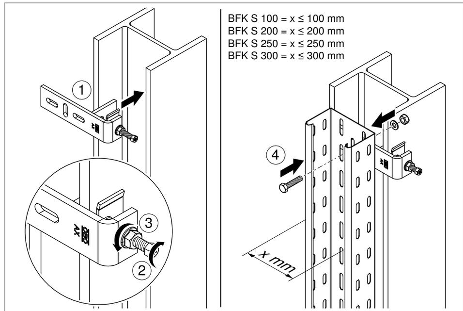
**Fig. 10:** Mounting a clamping piece on a vertical steel girder
