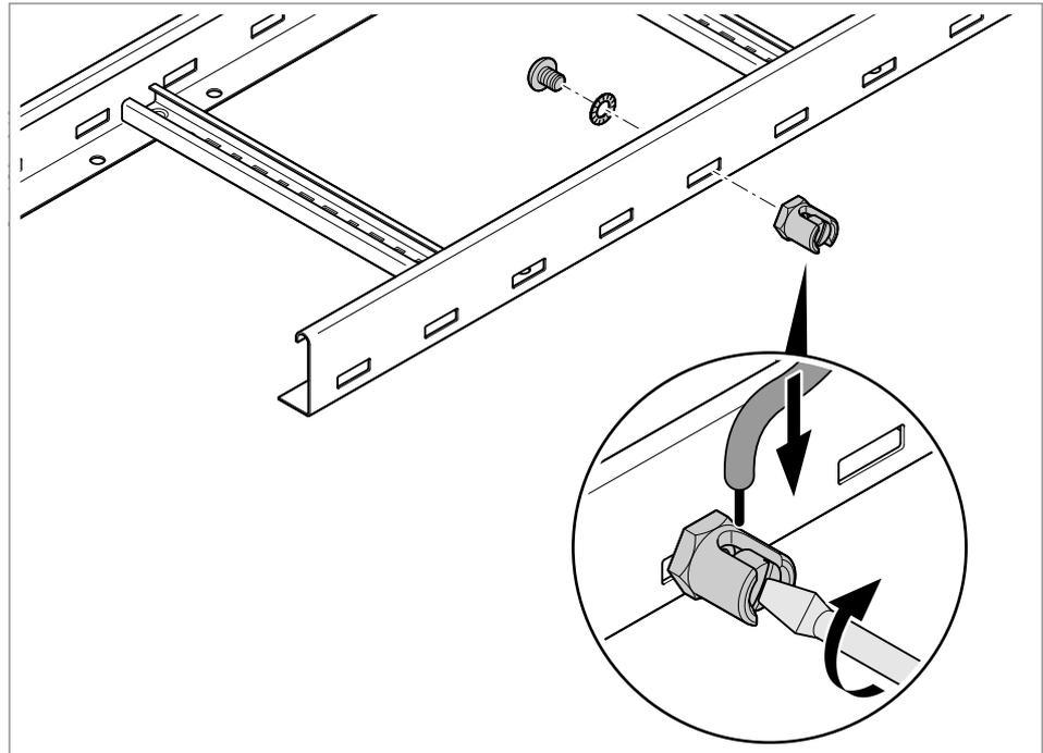
**Fig. 12:** Mounting the earthing terminal
