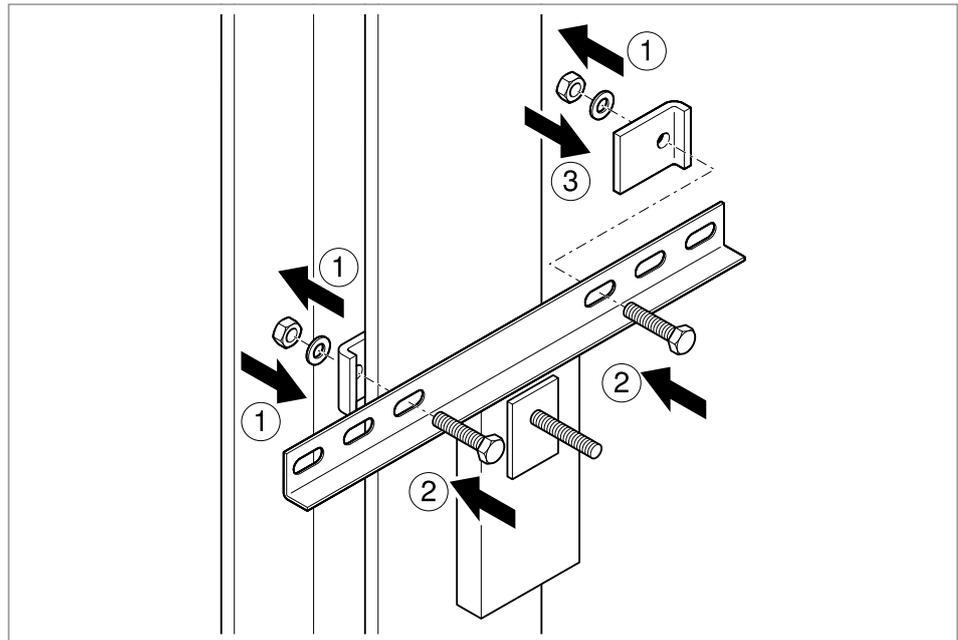
**Fig. 5:** Mounting a clamp fastening vertically
