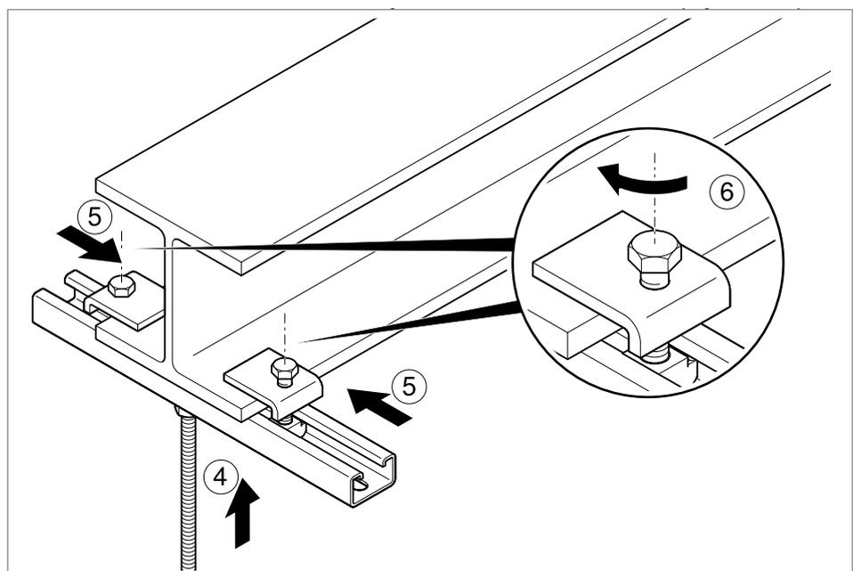
**Fig. 8:** Mounting a clamp fastening on a steel girder
