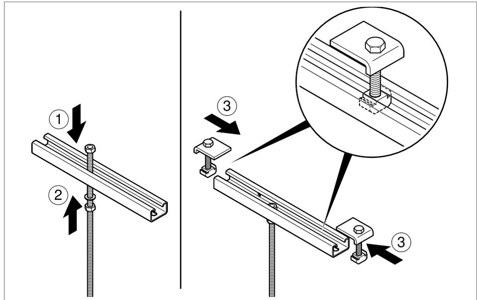
**Fig. 7:** Pre-assembling the centre suspension
