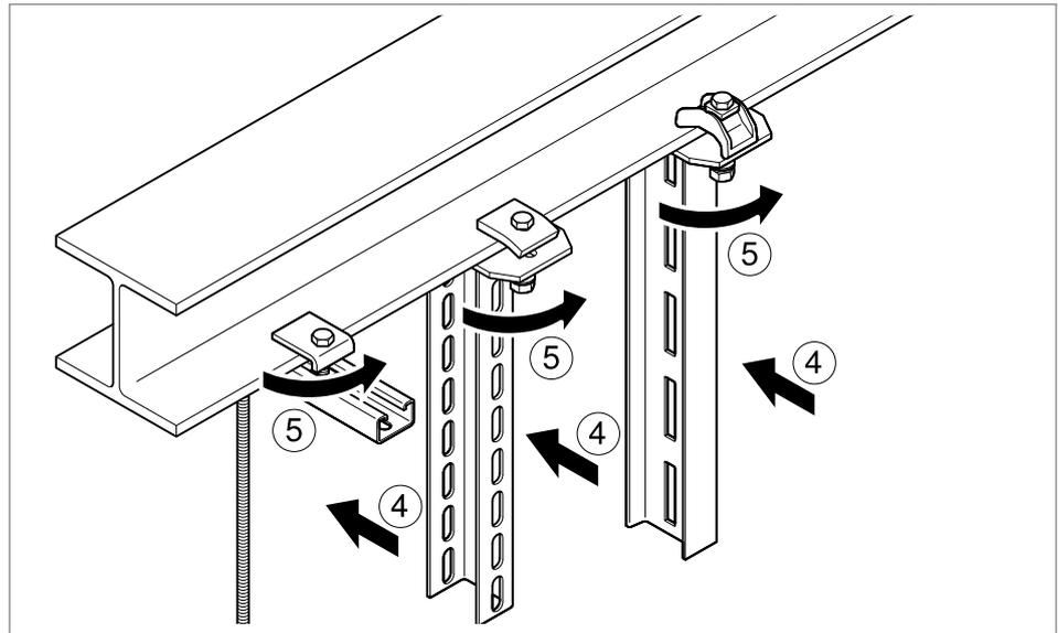
**Fig. 4:** Mounting a clamp fastening horizontally
