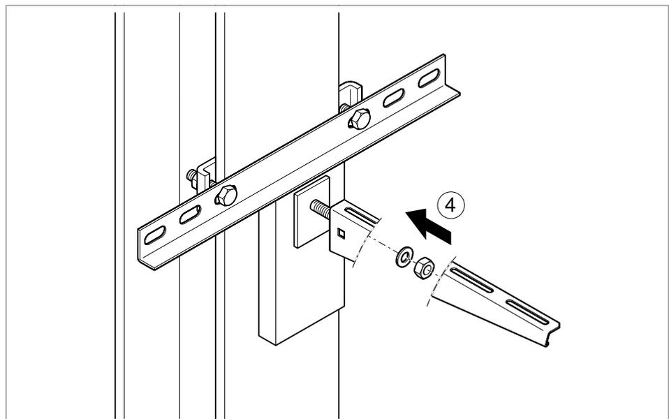
**Fig. 6:** Mounting the bracket
